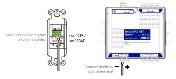
Note: When a long cable is used, it's recommended to run the cable separate from the speaker lines. A minimal distance on 12 inches between the speaker wires and the volume control cable is recommended.
